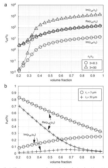
**Fig. 9.** Effective parameters as a function of volume fraction of particles *p*: (a) effective permittivity,  $r_1 = 5 \,\mu\text{m}$  and (b) effective permeability. Core conductivity  $\sigma = 5.8 \times 10^7 \,\text{S/m}$  and  $f = 2.45 \,\text{GHz}$ , shell thickness is 100 nm.
