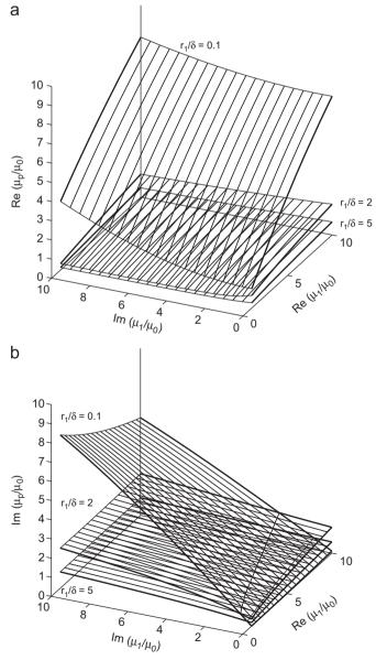
**Fig. 7.** Permeability  $\mu_p$  as a function of intrinsic permeability of the shell  $\mu_2$ , (a) real part and (b) imaginary part. Core is assumed to be nonmagnetic. To demonstrate the skin effect, ratio  $r_1/\delta$  is set to 0.1, 2 and 5. Within the used parameters the resultant  $\mu_p$  is a sum of the term depending on  $r_1/\delta$  ratio and the term depending on  $\mu_2$ .
