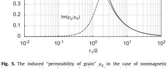
**Fig. 5.** The induced "permeability of grain"  $\mu_p$  in the case of nonmagnetic homogeneous particle as a function of  $r_1/\delta$  ratio. The result demonstrates that in spite of nonmagnetic material, the grains themselves show magnetic behavior.
