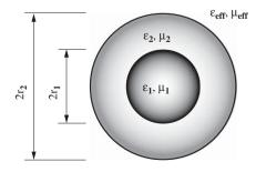
Fig. 2. Sketch of a coated particle.
