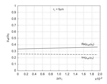
**Fig. 6.** Effect of the shell thickness on effective permeability  $\mu_{\rm eff}$  for  $r_1 = 5 \,\mu$ m, p = 0.9,  $\sigma = 5.8 \times 10^7 \,\rm S/m$  and  $f = 2.45 \,\rm GHz$ . The shell thickness  $\Delta r$  changes from 1 to 100 nm. For the presented parameters, the effective  $\mu_{\rm eff}$ , on the contrary to  $\varepsilon_{\rm eff}$ , is almost insensitive to the thickness of shell.
