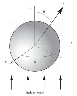
**Fig. 1.** Coordinate system used for calculation of scattered field. The *x*-polarized incident electromagnetic wave propagates along *z*-direction.
