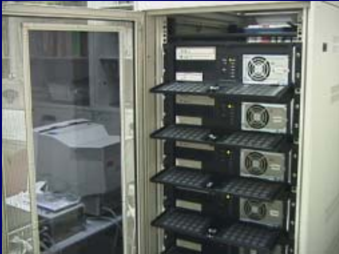
PC units mounted in a 19" rack
